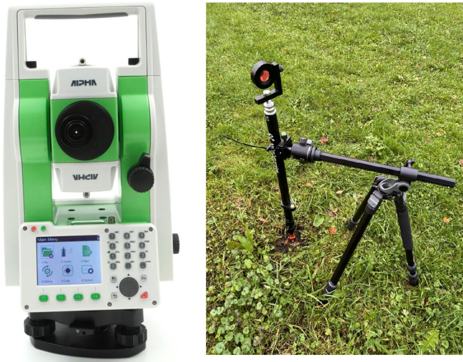
Image 4. Alpha Ti total station and measurement of reference points with a prism.
