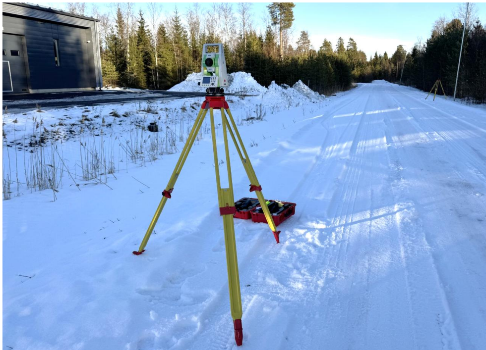
Figure 8. Alpha Ti total station used in a total station measurement on a Leica tripod and in the background a GMP104 prism on a similar tripod.
