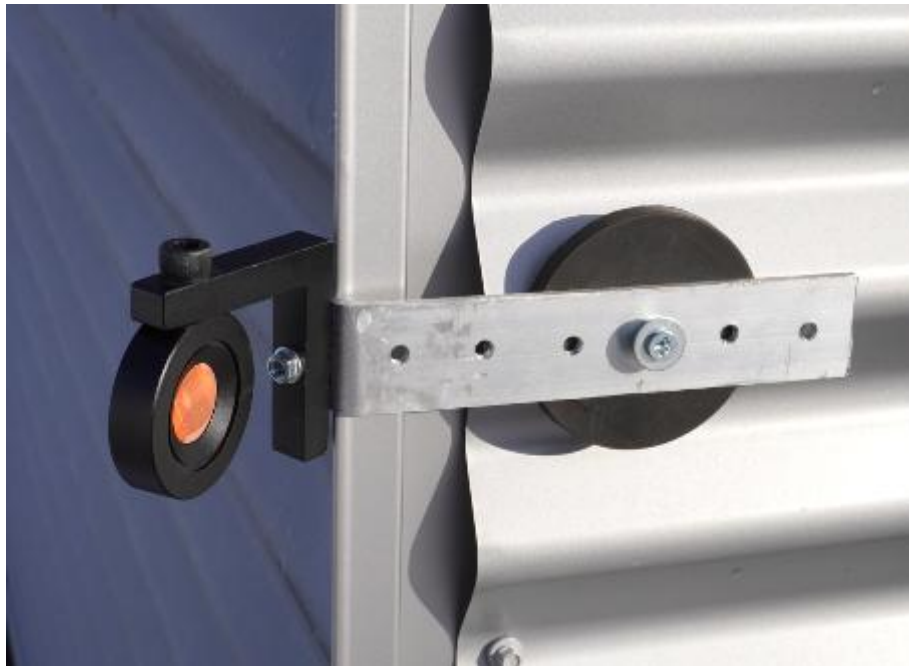
Figure 9. A GMP104 type prism used in a total station measurement and its magnetic attachment. The image also shows a metal corner strip.
