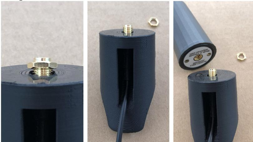
Image: Unscrewed nut before antenna installation.
