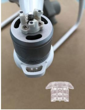
Image: Plastic clip removed from the Drone arm.
